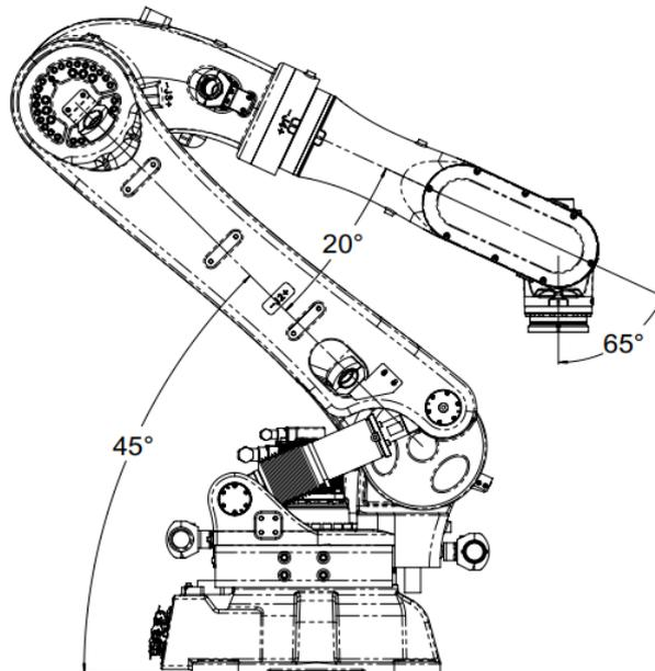
Figure 9-3 AIR220-3100/AIR130-3100/AIR170-3100 handling pose diagram
