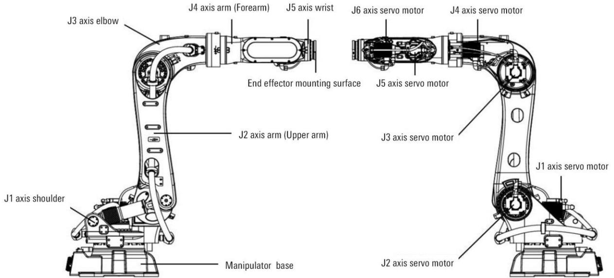
Figure 1-2 AIR280-2700/AIR130-2700/AIR170-2700/AIR220-2700 manipulator and its various parts
