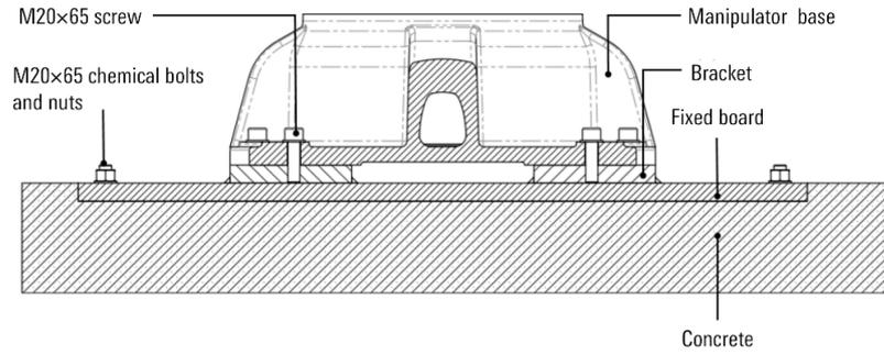
(b) Bracket fixation profile drawing
