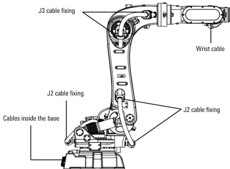
Figure 12-1 AIR280-2700/AIR130-2700/AIR170-2700/AIR220-2700 cable layout
