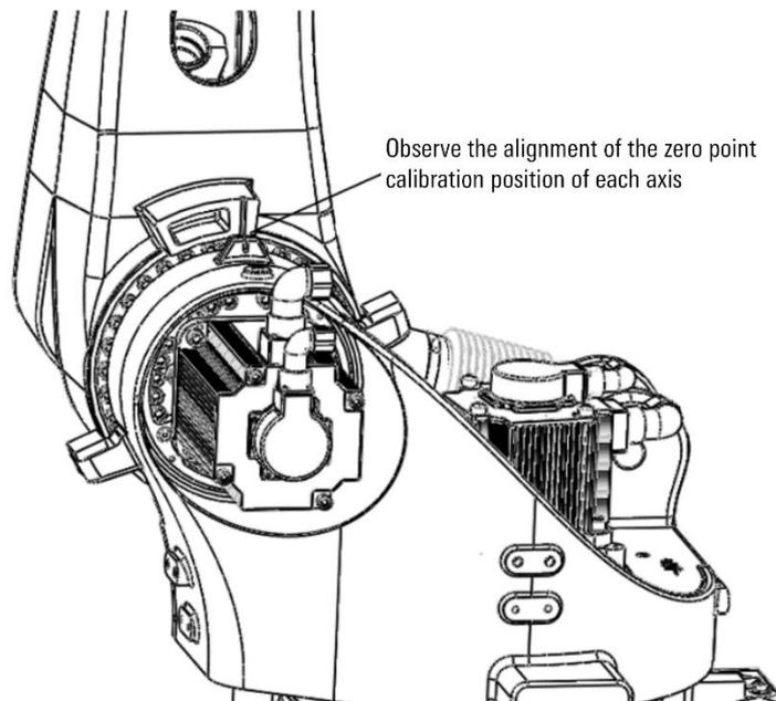
Figure 8-3 Large load manipulator naked eye zero point calibration method
