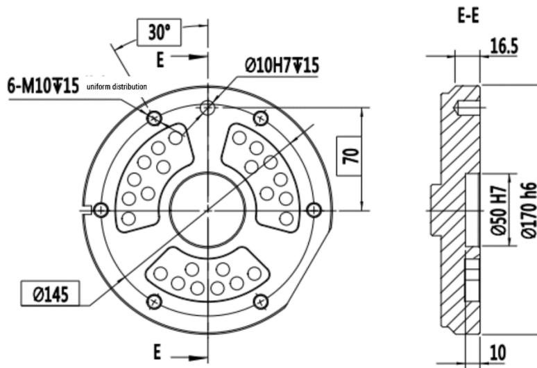
Figure 7-7 The flange dimension diagram of wrist
