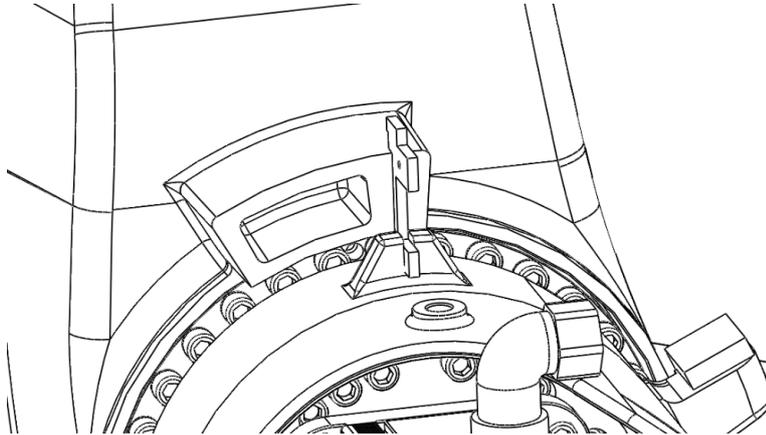
Figure 8-4 Large load manipulator zero point calibration block calibration method
