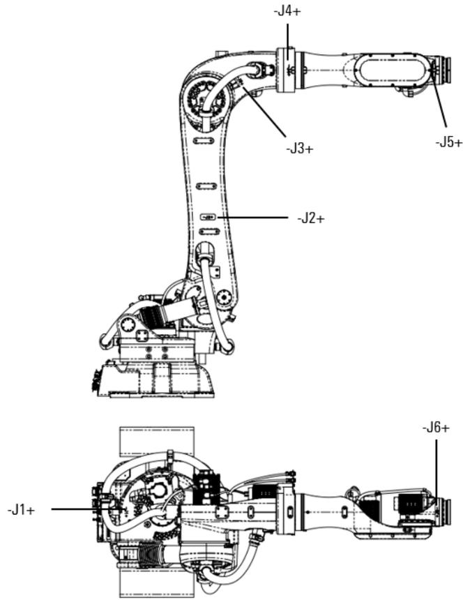
Figure 2-4 Direction identification of each axis on the AIR220-3100/AIR130-3100/AIR170-3100 manipulator
