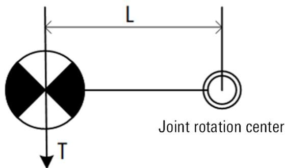
Figure 7-8 Diagram of load eccentricity
