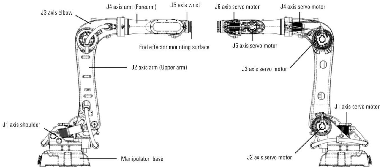
Figure 1-3 AIR220-3100/AIR130-3100/AIR170-3100 manipulator and its various parts
