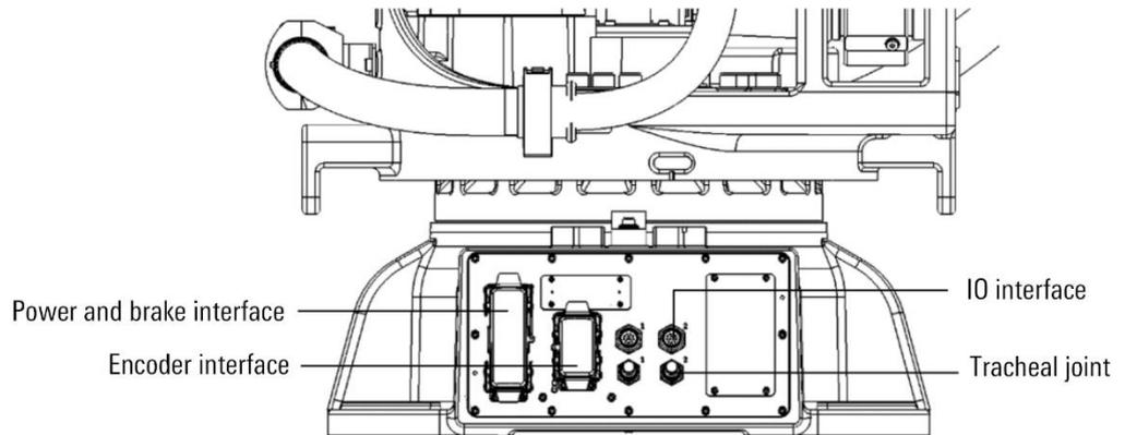
Figure 5-1 Electrical interface on the base of large load manipulator
