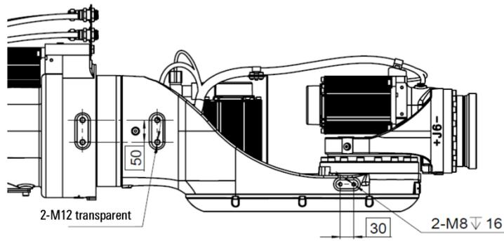
Figure 7-14 Dimensional diagram of the interface of the AIR280-2700/AIR130-2700/AIR170-2700/AIR220-2700's forearm
