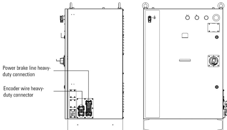
Figure 6-4 Control cabinet cable connector definition
