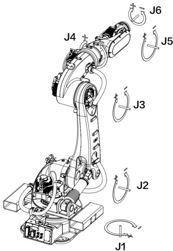
Figure 7-1 Movement direction of each axis of the AIR280-2700/AIR130-2700/AIR170-2700/AIR220-2700
