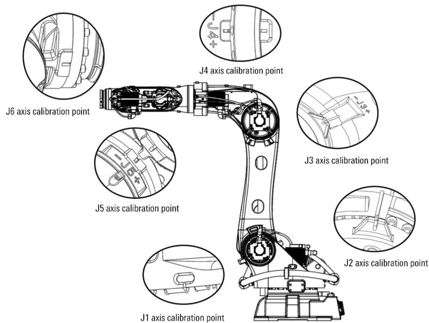
Figure 8-1 Diagram of zero points for each axis of AIR280-2700/AIR130-2700/AIR170-2700/AIR220-2700
