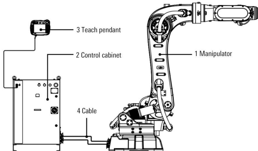
Figure 1-1 Composition of large load robot system
