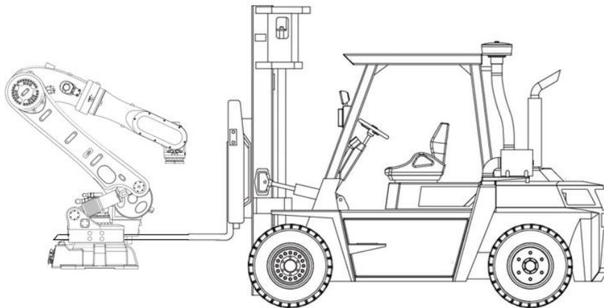
Figure 9-7 AIR220-3100/AIR130-3100/AIR170-3100 forklift handling diagram
