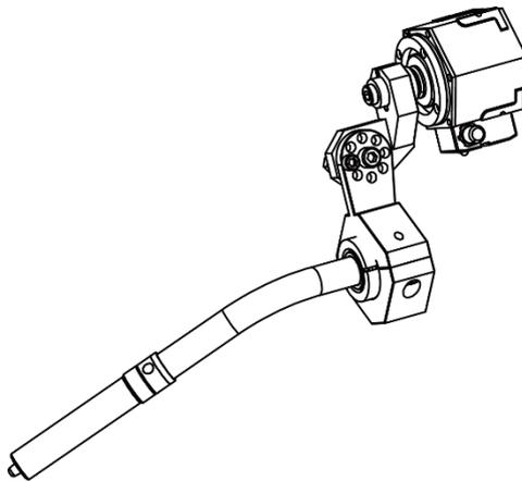
Figure 6-3 Arc welding gun for industrial robot
