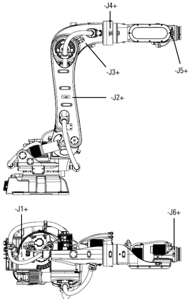
Figure 2-3 Direction identification of each axis on the AIR280-2700/AIR130-2700/AIR170-2700/AIR220-2700 manipulator
