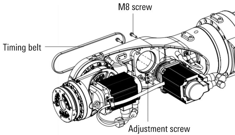
Figure 12-15 Remove timing belt
