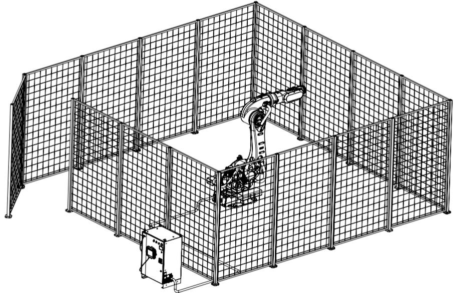
Figure 1 Diagram of safe work of industrial robots
