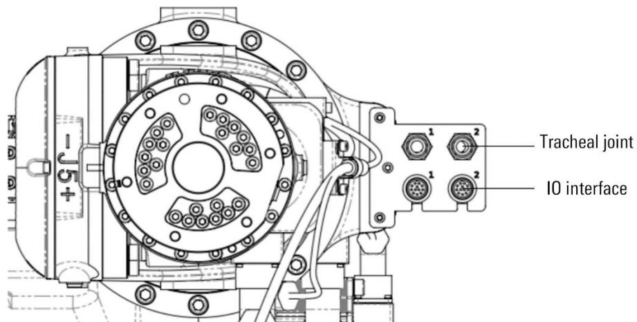
Figure 5-2 Electrical interface on the forearm of the large load manipulator
