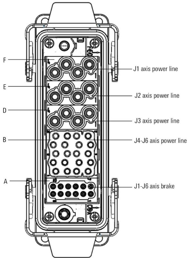
Figure 5-3 Large load manipulator power line heavy-duty connector
