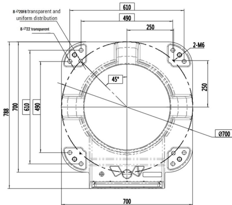
Figure 4-1 Manipulator base interface size
