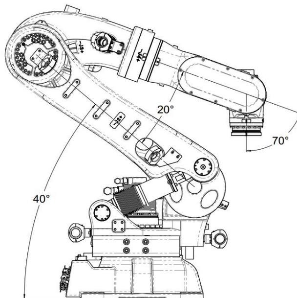
Figure 9-2 AIR280-2700/AIR130-2700/AIR170-2700/AIR220-2700 handling pose diagram
