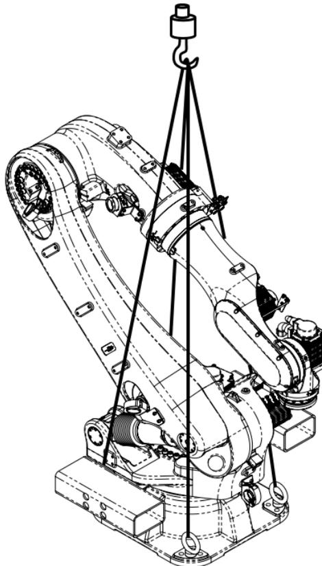
Figure 9-9 AIR220-3100/AIR130-3100/AIR170-3100 lifting ring handling diagram
