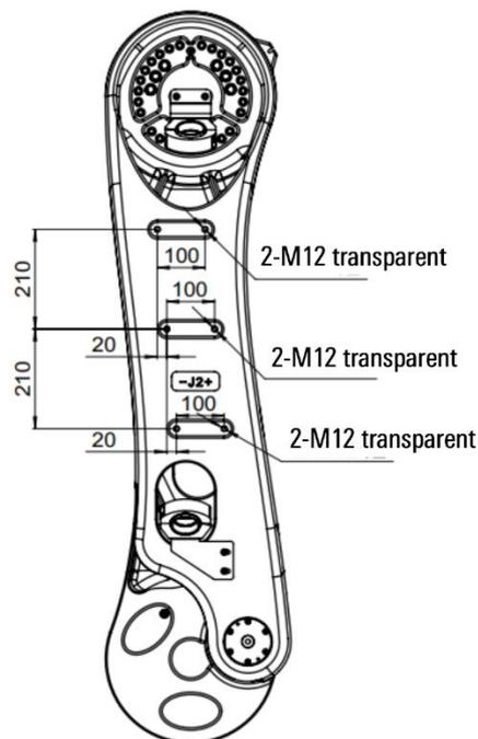
Figure 7-16 AIR280-2700/AIR130-2700/AIR170-2700/AIR220-2700 upper arm interface dimension diagram
