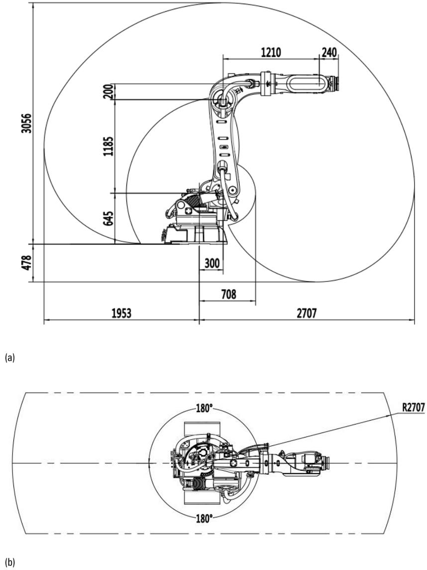
Figure 7-3 Operating range of the AIR280-2700/AIR130-2700/AIR170-2700/AIR220-2700
