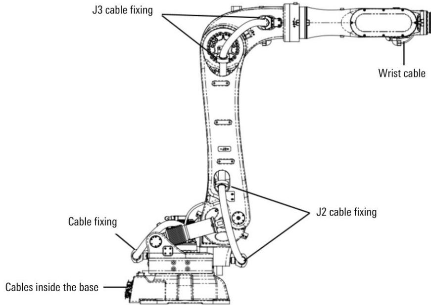
Figure 12-2 AIR220-3100/AIR130-3100/AIR170-3100 cable layout
