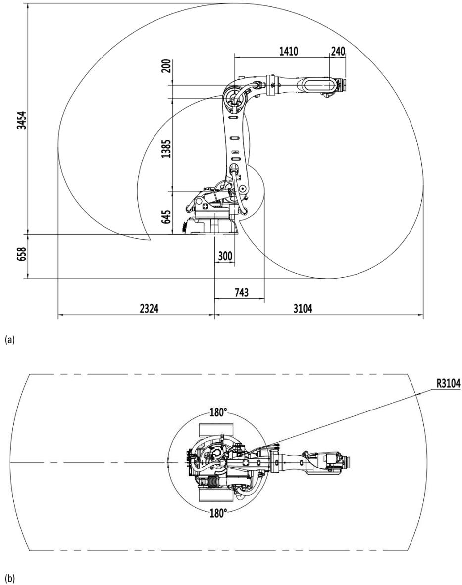
Figure 7-4 Operating range of the AIR220-3100/AIR130-3100/AIR170-3100
