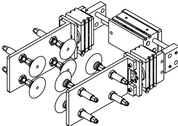
Figure 6-2 Suction cups for industrial robots
