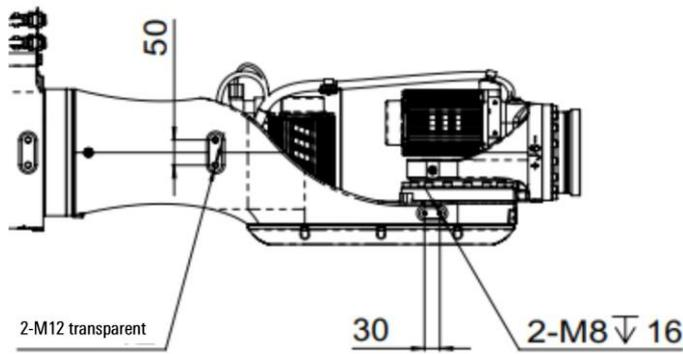
Figure 7-15 Dimensional diagram of the interface of the AIR220-3100/AIR130-3100/AIR170-3100's forearm
