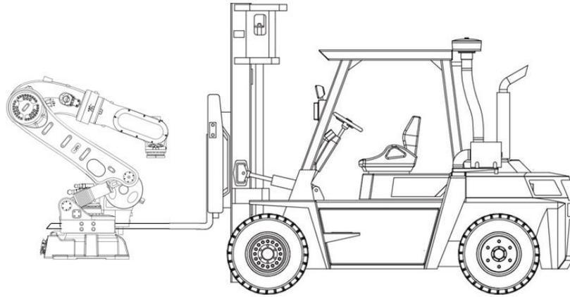
Figure 9-6 AIR280-2700/AIR130-2700/AIR170-2700/AIR220-2700 forklift handling diagram
