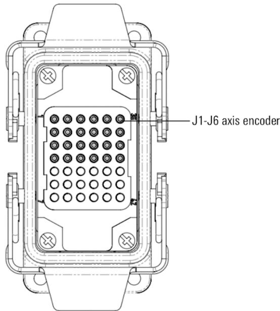
Figure 5-4 Large load manipulator encoder line heavy-duty connector
