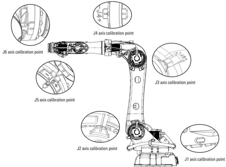
Figure 8-2 Diagram of zero points for each axis of AIR220-3100/AIR130-3100/AIR170-3100
