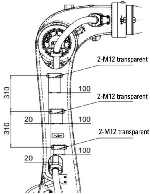
Figure 7-17 AIR220-3100/AIR130-3100/AIR170-3100 upper arm interface dimension diagram
