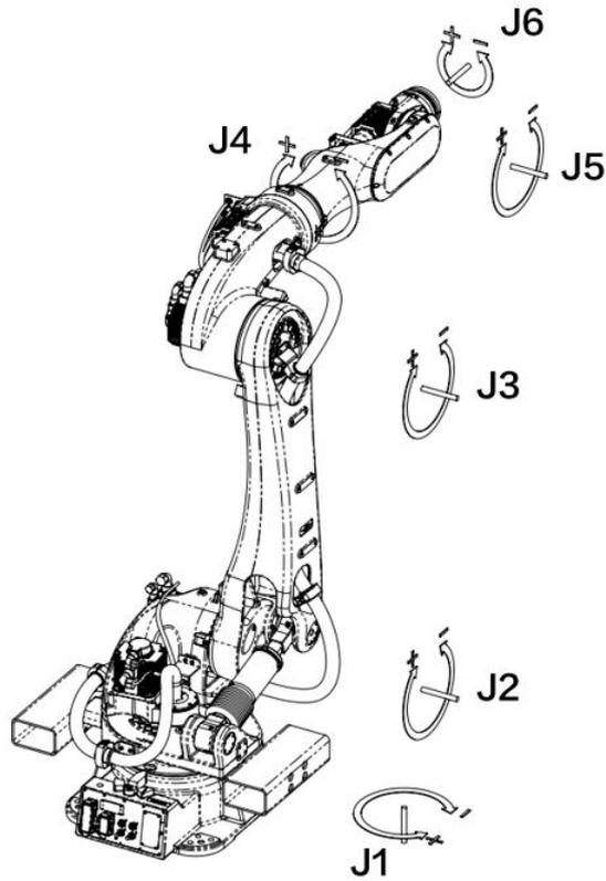
Figure 7-2 Movement direction of each axis of the AIR220-3100/AIR130-3100/AIR170-3100
