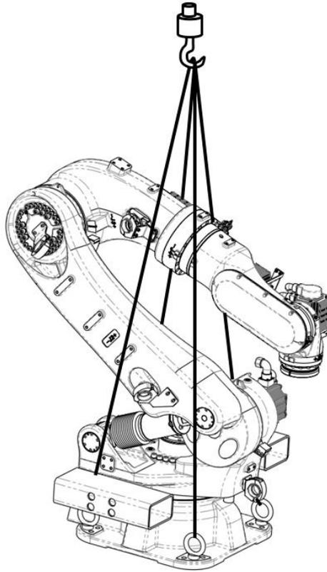
Figure 9-8 AIR280-2700/AIR130-2700/AIR170-2700/AIR220-2700 lifting ring handling diagram
