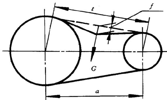
Figure 12-16 Timing belt installation deflection
