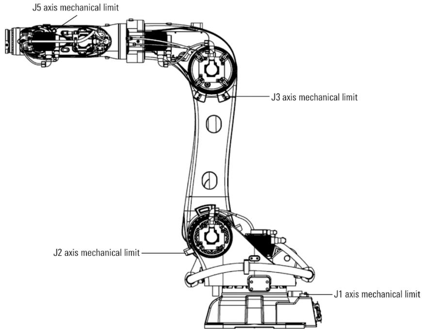
Figure 7-5 Mechanical brakes on the AIR280-2700/AIR130-2700/AIR170-2700/AIR220-2700
